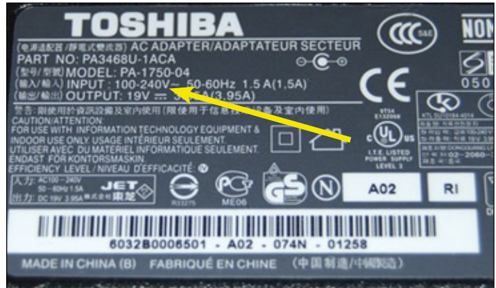
Before plugging an item in, ensure it is 220-230 volt capable.
